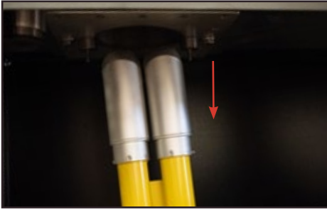
5 - Remove the burner from its housing
