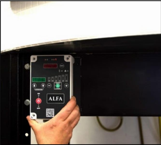
**2 -** Once the burner is in place attach the control unit to the base crossbar using self-drilling screws or a drill
